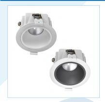
A fixed recess-mounted LED waterproof downlight with a deep anti-glare design, die-cast aluminum body, and efficient heat sink. Finished in sandy white powder coating, it features an anti-glare lens for comfortable, high-quality illumination.
